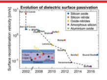
In order to continue to decrease cost and improve performance of silicon solar cells it is essential to minimize electrical losses due to the recombination of electron-hole pairs at cell surfaces. The most common approach is the application of a dielectric coating to suppress these losses, which occur via a combination of different mechanisms. This review article examines the range of dielectric coatings developed in the last two decades and how these coatings act to increase cell performance.
