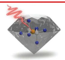
The silicon vacancy color center, an atom-sized defect in diamond, has recently emerged as a promising tool for solid-state-based quantum technologies, due to its favorable optical properties. In this review, the authors summarize the center's electronic and optical properties, as well as recent advances in controlling its quantum state, making it accessible for future quantum information processing applications.
