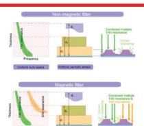
Both nanoscale nonmagnetic and magnetic graphene hybrid fillers have been prepared as the effective absorbers, suggesting that a combination of developing microscopic dielectric-magnetic coupled absorbers and macroscopic structure design would fundamentally extend the effective absorption bandwidth of the electromagnetic absorption materials.
