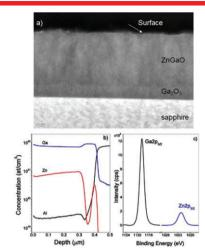
Alema et al. grew doped (Zn) and undoped  $\beta$ -Ga<sub>2</sub>O<sub>3</sub> epitaxial films using MOCVD and fabricated the films into MSM photodetectors. The Zn doped  $\beta$ -Ga<sub>2</sub>O<sub>3</sub> detectors showed a peak responsivity of 210 A/W with a rejection ratio of 5 × 10<sup>4</sup>. The results provide a roadmap towards achieving high responsivity SBPs with strong selectivity in the solar blind spectral window.
